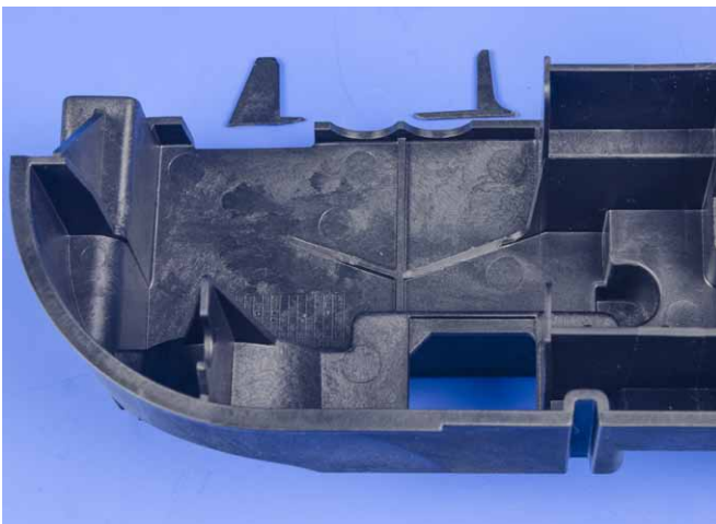
Rear frame with support ribs removed
