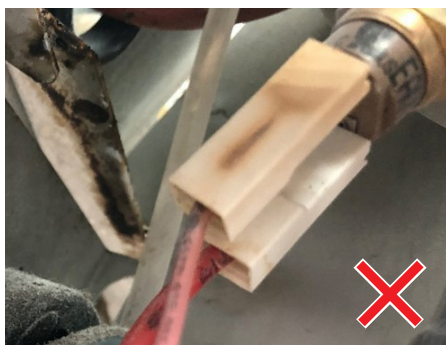
Defective, bent plug-in connector
