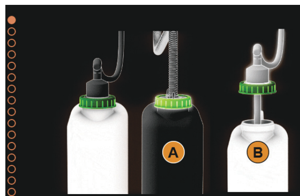
Fig.: Cleaning programme with external drinking/waste water tank
